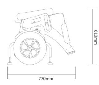
Max.Load 90kg Suitable Height 1.5m~2.1m Max. Speed 6-9km/h Applicable Temperature -10°C~40°C Charge Time 520Wh/about 180min Charge Voltage AC100-240V 50-60Hz
